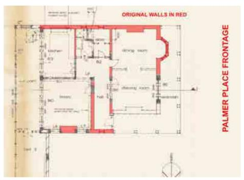
Figure 6: 1987 architect's documents showing ground floor demolition plan, showing retained walls in red
